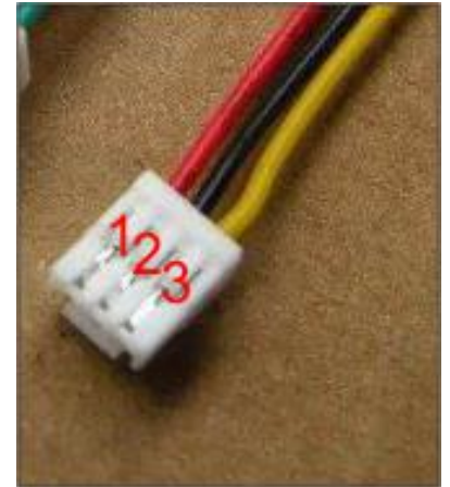
RS232: 3p GH with lock socket(GH 1.25mm)
