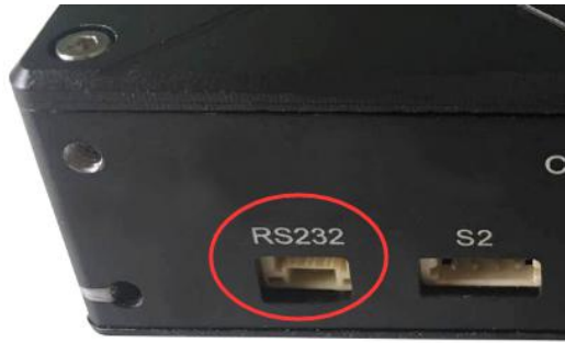
RS232: 3p GH with lock socket(GH 1.25mm)
